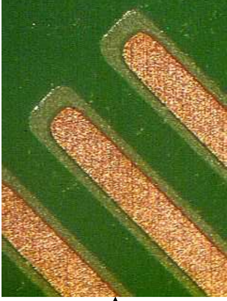
Original Pad 18 \mu m Copper
