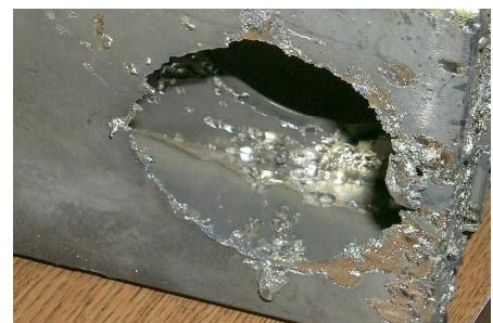
Figure 2. Erosion of stainless steel wave
